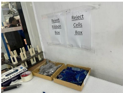
Figure 6.7: Defective Cells and Ribbons
